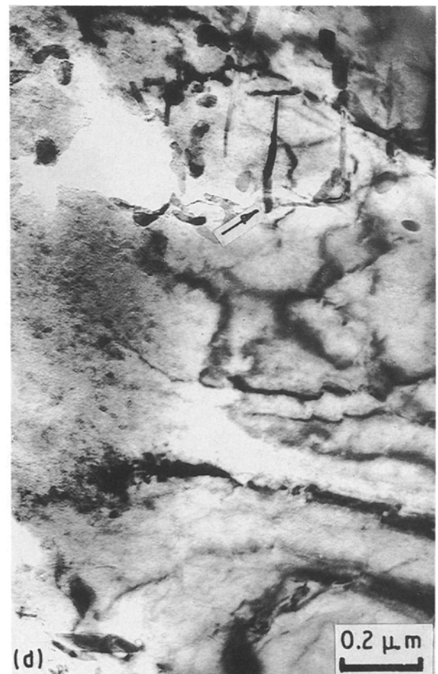
Figure 4 (a) Transmission electron micrograph showing bainite and ferrite in steel A in austenitized and argon-cooled condition; (b) transmission electron micrograph showing the presence of bainite and ferrite in steel B in austenitized and argon-cooled condition; (c) SAD pattern from the carbides shown in (b) confirming the presence of cementite with \langle \bar{1}11 \rangle zone axis; (d) transmission electron micrograph showing presence of fine needle-like precipitates in the ferrite region of steel B in argon-cooled condition.
